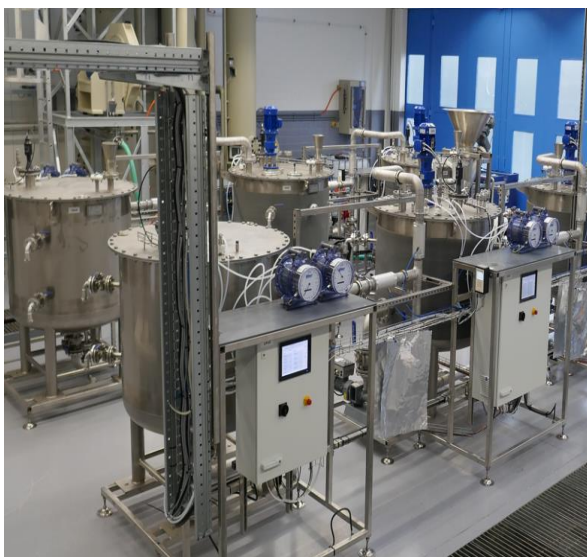
Figure 2: Complex biogas test plant equipped with 6 stations using 1,000 l stainless steel bioreactors – installed at the University of Münster/Germany.
